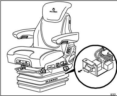
If a power-consuming element fails, the internal safety system should be checked first.
